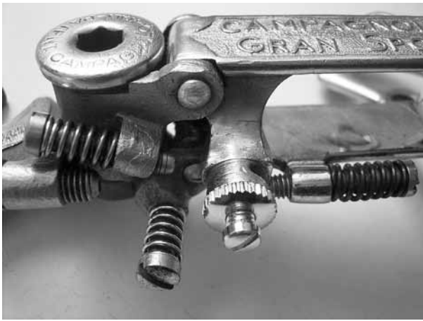
Fig. 3: Detail of the Gran Sport 51-1: The cable clamp bolt swivels to prevent bending the cable. The "additional" screw adjusts how far the derailleur can swing.
