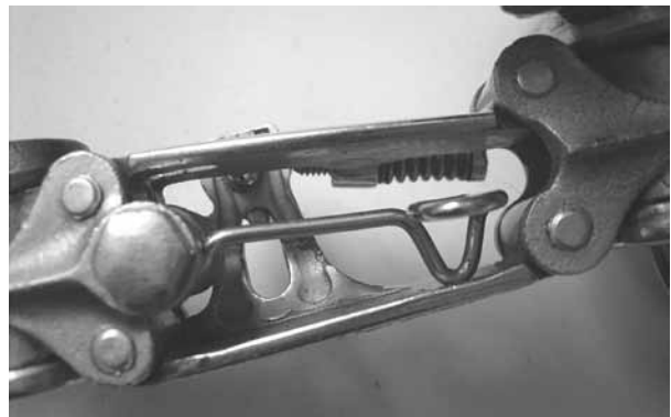
Fig. 9: Model 52-1: The plates were domed and angled instead of parallel, to make them stiffer. The rib has been deleted.
