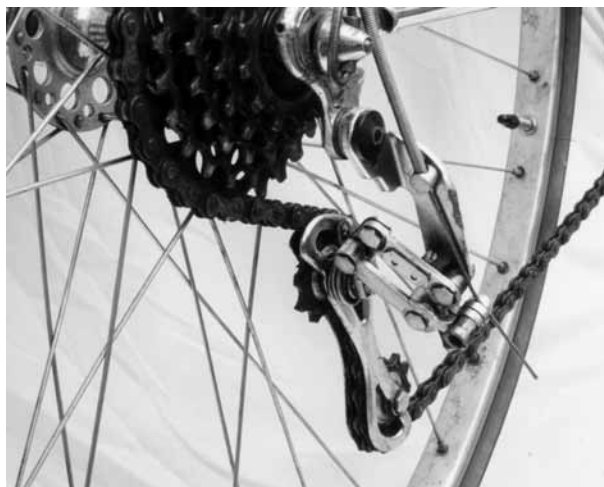
Huret turned the Nivex parallelogram downward for the Allvit, combining the advantages of Campagnolo (easy wheel removal, easy set-up) and Nivex (constant chain gap). (Second version on 1960 René Herse racer).
