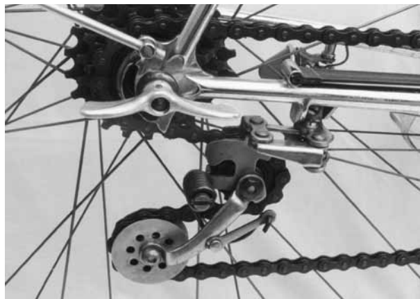
Nivex cyclotouring derailleur (1962 Singer randonneur). The dropout incorporates a chainrest to facilitate wheel removal. The two shifter cables exit on the right.
