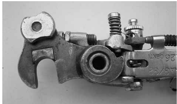
Fig. 4: The "additional" screw limits the derailleur swing (51-1). The oblong hole holds the end of the return spring.
