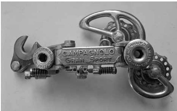
Fig. 8: The extra-large pulley cage was used only in 1952. The parallelogram geometry has been finalized already. (Model 52-1)
