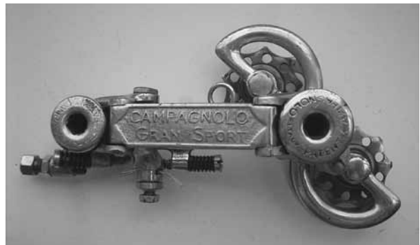
Fig. 7: Model 51-3 (shown) is identical to 51-2, except for different screws and bolts. The "additional" screw is gone.
