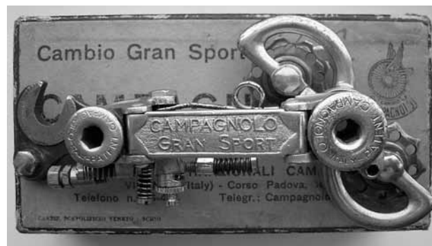
△ Fig. 2: The first production model (51-1) of the Gran Sport derailleur was much modified from the prototype. A return spring simplifies installation (with only one cable). Limit screws facilitate setup. The numerous adjustment screws were simplified over time.
