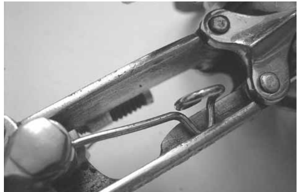
Fig. 5: Reinforcement rib found only on 51 models.
