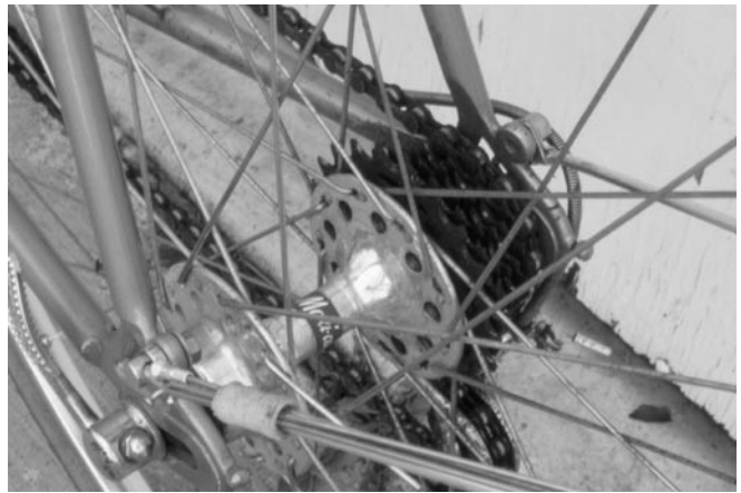
△ Compromises on the Rivendell: Horizontal dropouts don't work well with fenders. Also, the eyelets are not offset toward the outside, so there is no space for a nut between the eyelet and the chain on the smallest cog, as needed for an eyebolt attachment. Maxi-Car hubs allow spoke replacement without freewheel removal. Three spare spokes are carried on the fender stay.
