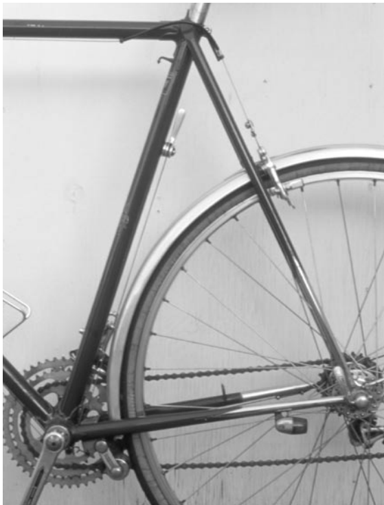
△ Integrated lighting on a true randonneur bike (1990 Alex Singer): BB generator controlled by shift lever on seat tube, rear light under chainstay. Internal wires. Vertical dropouts facilitate wheel removal with fenders.
